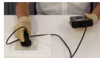
Non-destructive probe (Eddy current method)
